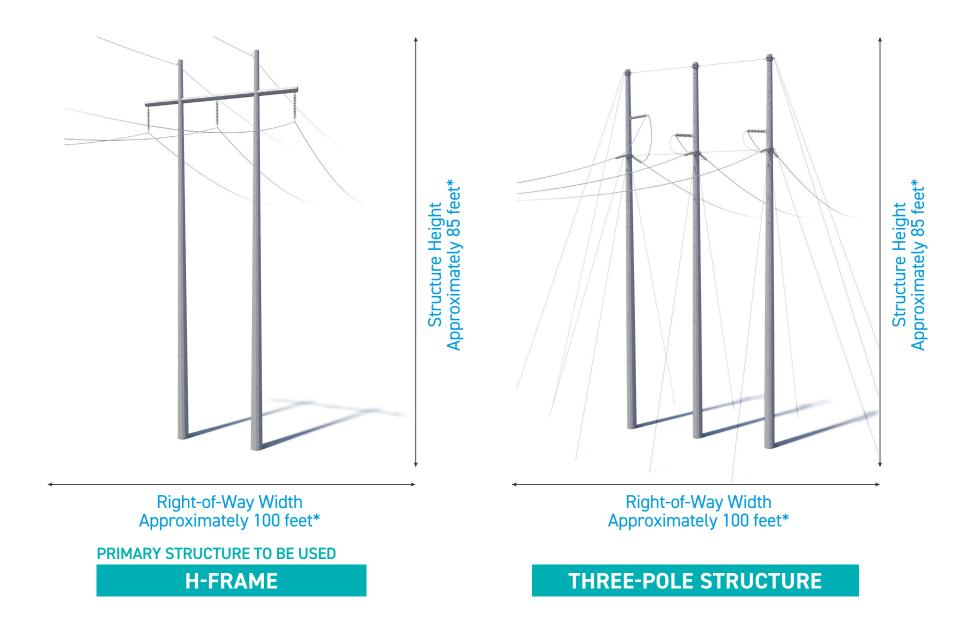
Crews plan to rebuild the line using mainly steel H-frames or three-pole structures depending on final engineering.
